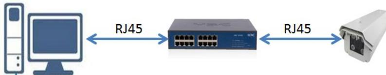
Once the network and power are connected, check that the LEDs on the switch port start to light up. flashing. This means the camera is working and you can continue IP address configuration. For convenience, the camera also has two network LEDs on the network connector so you can check the proper functioning of the communication even from the camera side.
